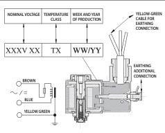
The coil 3009M Exm is developed to fit Amisco operators. If a different operator is used, make sure that the coil powered with nominal voltage does not show a power consumption exceeding the values mentioned above.
